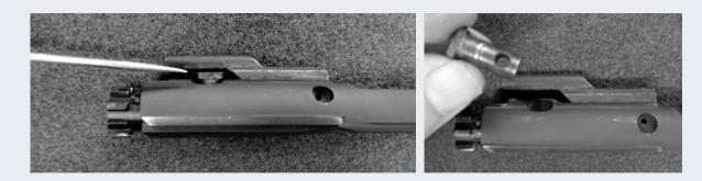
**12**. Remove the bolt from the bolt carrier body.
