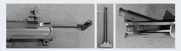
8. To field strip the bolt, make sure that the bolt is in the forward or extended position. only go through one side of the bolt carrier.)
