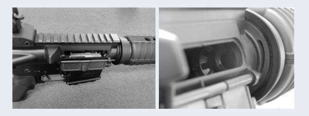
www.franklinarmory.com FRANKLIN ARMORY® 31 Warning: Do not closely peer into the ejection port when clearing a mis-feed. If a cartridge primer were to be struck by a hard object such as another cartridge, the primer could ignite causing a case head rupture. A case head rupture could cause severe injury or death to you or others around you.
