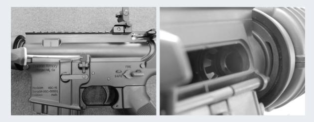
4. Push the takedown pin on the left side so that it will slide out to the right side. The pin is designed to stop its travel just short of falling completely out. This action, when completed, will allow the upper receiver to pivot forward.
