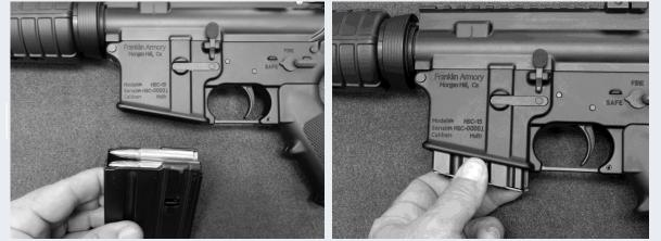
8. Drop the bolt carrier by depressing the upper portion of the bolt catch while keeping the muzzle pointed in a safe direction. This activity will automatically strip the top live round off of the magazine and chamber the round. Keep the firearm safety selector lever on "Safe" until you are ready to fire.
