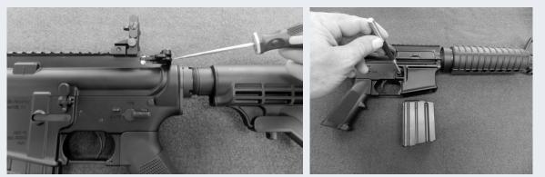
4. Remove the ammunition source by removing the magazine. To do so, depress the magazine release button and pull the magazine out the bottom of the magazine well.
