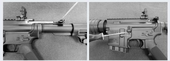
2. Push the charging handle forward until it snaps back into position.
