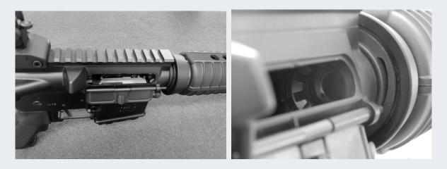
5. Look through the ejection port to the inside of the chamber. Verify that there is not a round of ammunition in the chamber.
