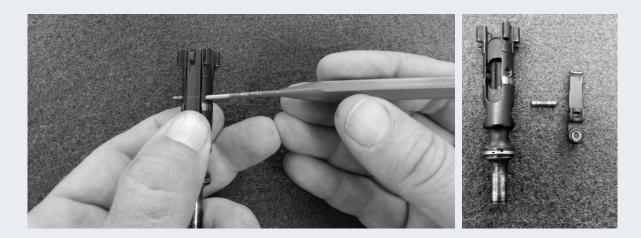
14. Do not attempt to remove the rubber grommet from the extractor spring.
