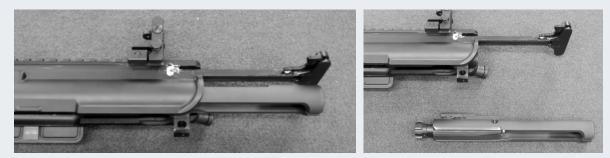
7. Remove the charging handle by sliding the charging handle to the point where the "ears" (or protruding tabs) on the charging handle can slip through the keyway on the upper receiver. When the charging handle is extended out approximately 4.4" from the upper receiver, the ears on the charging handle should be lined up and can slide up through the keyway.
