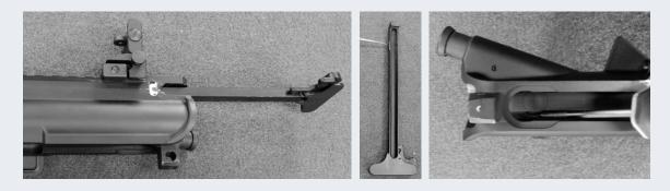
8. To field strip the bolt, make sure that the bolt is in the forward or extended position. Next remove the firing pin retaining pin. (It looks like a cotter pin and is designed to only go through one side of the bolt carrier.)
