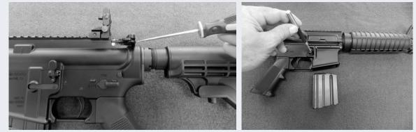
4. Remove the ammunition source by removing the magazine. To do so, depress the magazine release button and pull the magazine out the bottom of the magazine well.
