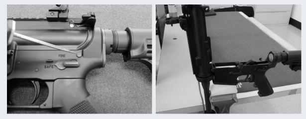
**Warning:** Never dry fire the firearm when the upper and lower are not fully assembled. The steel hammer will hit the rear of the aluminum magazine well and eventually cause it to crack.
