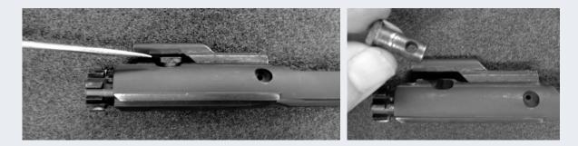
**12**. Remove the bolt from the bolt carrier body.
