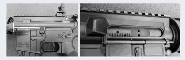
**Warning:** Do not carry your firearm with the bolt carrier locked back while a loaded magazine is locked into the magazine well. If the bolt carrier were to get jostled and slide forward, an accidental discharge may result, especially if the safety selector is not set on "Safe."
