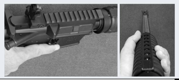
8. Drop the bolt carrier by depressing the upper portion of the bolt catch while keeping the muzzle pointed in a safe direction. This activity will automatically strip the top live round off of the magazine and chamber the round. Keep the firearm safety selector lever on "Safe" until you are ready to fire.
