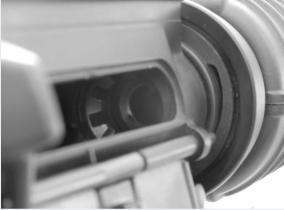
5. Look through the ejection port to the inside of the chamber. Verify that there is not a round of ammunition in the chamber.
