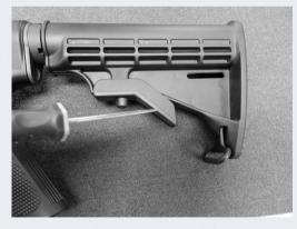
This collapsible buttstock is designed to have tolerance to allow for operation if fouled by small amounts of sand or dirt. However, from time to time the collapsible buttstock may require cleaning in order to function properly.
