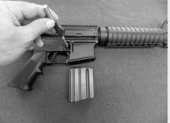
4. Remove the ammunition source by removing the magazine. To do so, depress the magazine release button and pull the magazine out the bottom of the magazine well.
