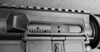
**Warning:** Do not carry your firearm with the bolt carrier locked back while a loaded magazine is locked into the magazine well. If the bolt carrier were to get jostled and slide forward, an accidental discharge may result, especially if the safety selector is not set on "Safe."
