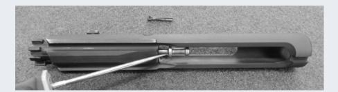
10. After cleaning, use a high quality firearms specific lubricant to lightly coat the external parts. A quality "dry lube" is recommended for the exterior metal surfaces. In any case, do not leave any obvious finger prints on the metal surfaces as finger moisture may lead to corrosion.
