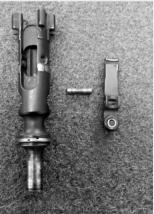
14. Do not attempt to remove the rubber grommet from the extractor spring.
