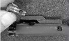
12. Remove the bolt from the bolt carrier body.
