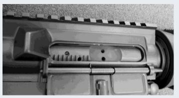
**Warning:** Do not carry your firearm with the bolt carrier locked back while a loaded magazine is locked into the magazine well. If the bolt carrier were to get jostled and slide forward, an accidental discharge may result, especially if the safety selector is not set on "Safe."
