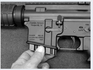
8. Drop the bolt carrier by depressing the upper portion of the bolt catch while keeping the muzzle pointed in a safe direction. This activity will automatically strip the top live round off of the magazine and chamber the round. Keep the firearm safety selector lever on "Safe" until you are ready to fire.
