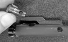
12. Remove the bolt from the bolt carrier body.
