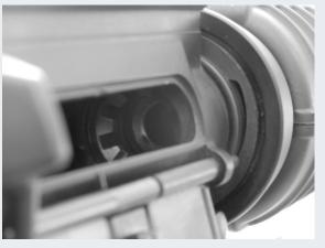
5. Look through the ejection port to the inside of the chamber. Verify that there is not a round of ammunition in the chamber.
