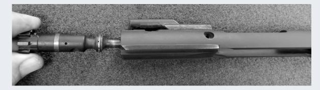
13. Push on the back of the extractor to relieve pressure off of the extractor roll pin.
