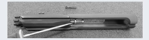
11. Turn the bolt cam pin 90 degrees and remove it from the carrier.
