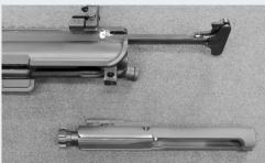
6. Remove the charging handle by sliding the charging handle to the point where the "ears" (or protruding tabs) on the charging handle can slip through the keyway on the upper receiver. When the charging handle is extended out approximately 4.4" from the upper receiver, the ears on the charging handle should be lined up and can slide up through the keyway.
