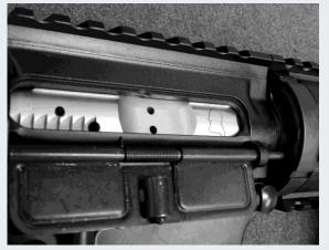
Warning: Never allow a finger to enter the ejection port while the bolt catch is depressed. The bolt carrier will slide forward with considerable force.
