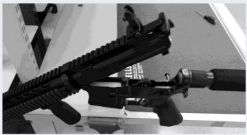
**Warning:** Never dry fire the Pistol when the upper and lower are not fully assembled. The steel hammer will hit the rear of the aluminum magazine well and eventually cause it to crack.
