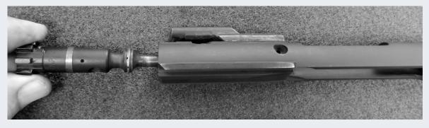
13. Push on the back of the extractor to relieve pressure off of the extractor roll pin. Use an appropriately sized punch to remove the roll pin.
