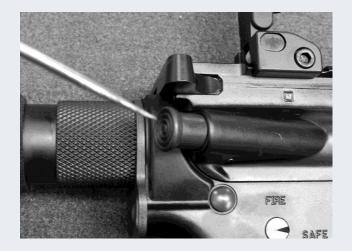
Warning: The force necessary to articulate the forward assist is slight. If it takes significant force to push the forward assist button, stop what you are doing and disassemble the firearm to diagnose why the firearm is not operating correctly. Often dirt, fouling, or improper ammunition may be the cause. Make sure that the chamber is not in any way encumbered before proceeding.
