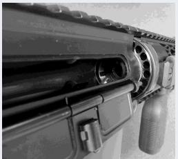
Look through the ejection port to the inside of the chamber. If there is a live round in the chamber area, you will need to drop the magazine free from the firearm. Now that the magazine is clear, check to see if there is a round in the chamber and remove as necessary.
