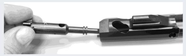
12. Push on the back of the extractor to relieve pressure off of the extractor roll pin. Use an appropriate sized punch to remove the roll pin.
