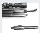
6. Remove the charging handle by sliding the charging handle to the point where the "ears" (or protruding tabs) on the charging handle can slip through the keyway on the upper receiver. When the charging handle is extended out approximately 4.4" from the upper receiver, the ears on the charging handle should be lined up and can slide up through the keyway.
