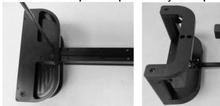
I. Unscrew the  $\frac{1}{4}$ -28-1" Grip Screw from the Lower Receiver Extension and AR15 Receiver.
