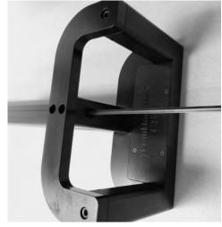
B. If your CSW™ is attached to a firearm, unscrew the singular ½-28-1" screw that attaches the Column Block to the Receiver Extension with a 3/16" Allen Wrench.
