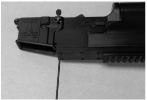
D. Unscrew the two 6-32- $\frac{1}{2}$ " screws holding the Left Side Plate with a 7/64" Allen Wrench, and set the screws and Side Plate aside.
