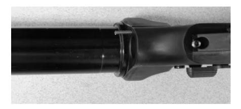
E. Slide the Clam Shells over the Receiver Extension and compress the takedown Pin Detent Spring.
