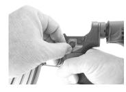
while in Binary Mode. Please note that if the operator should pull the Trigger back prior to reset, the Hammer will not be released when the Trigger is pulled. However, when the Trigger is subsequently released, the Hammer will be allowed to fall to the Firing Pin. Consequently, it is recommended that BFS III™ operators use a "pull through, release through" technique.
