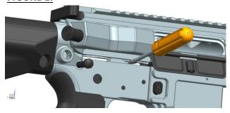
Be careful to not pull the Upper and Lower apart so tightly that it binds the Carrier in between the two as this may prevent the Carrier from moving forward even if the Hammer is appropriately clear of the Carrier. In addition, be careful not to mar the finish of the Upper or Lower Receiver.
